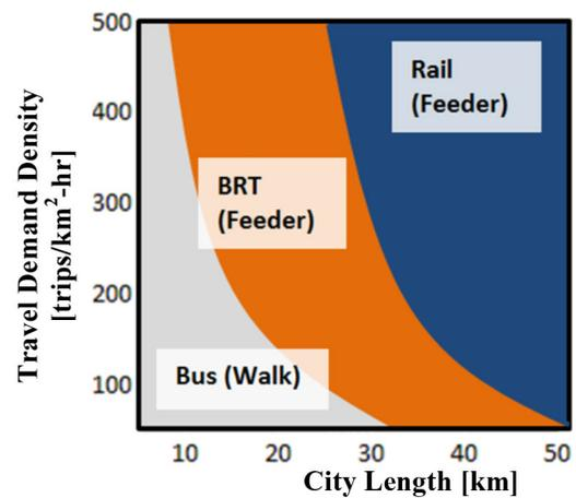
Figure 3. Most Cost-Effective Transit Technology Feeder Bus Access to Bus Rapid Transit and Rail
