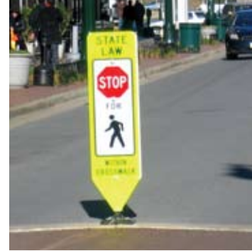
“In-roadway pedestrian crossing signs” can increase the percentage of drivers who yield to pedestrians in crosswalks.
