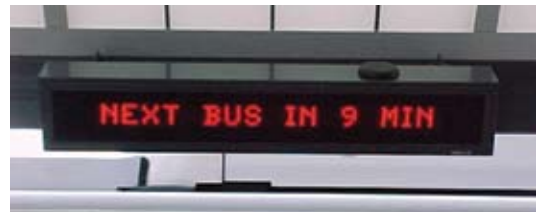
This real-time information sign counts down the time until the arrival of the next bus on Los Angeles' Metro Rapid system.
