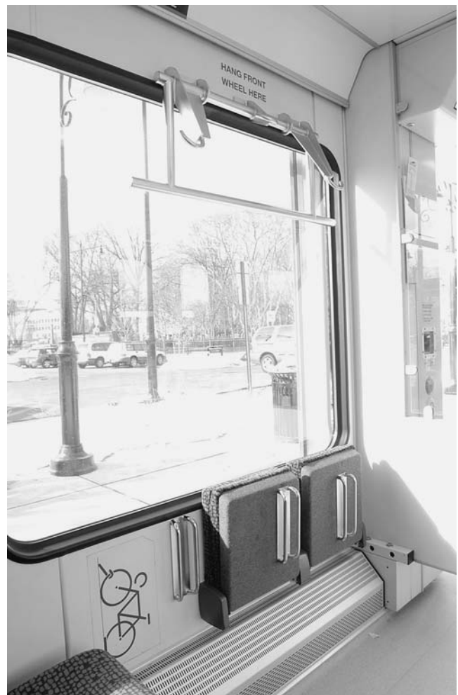
FIGURE 18 New Jersey Transit Corp. provides hooks for hanging bicycles on its River LINE light rail service.
