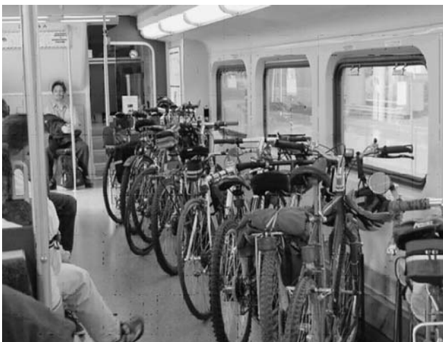
FIGURE 17 Altamont Commuter Express allows space for an additional two to four bicycles as overflow on remaining rail cars.
