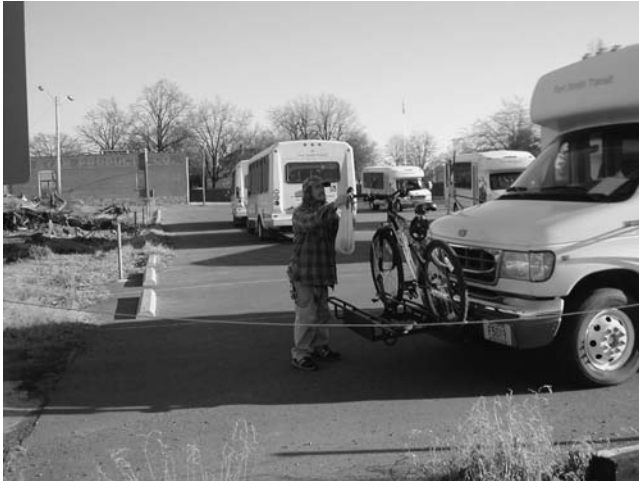
FIGURE 13 Easy-to-use, one bar lock, front-mounted bike rack—Fort Smith Transit.
