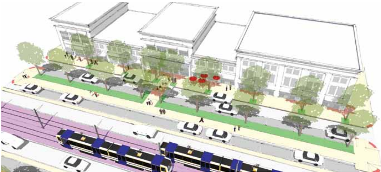
Single row of parallel parking, and one-way drive lane.
